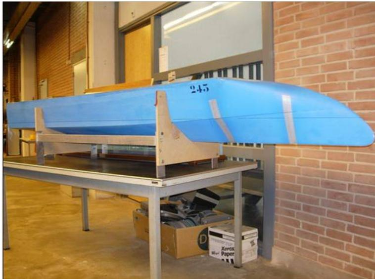
**Figure 5b: Model according to the Wave Piercer Concept (WPC)**
