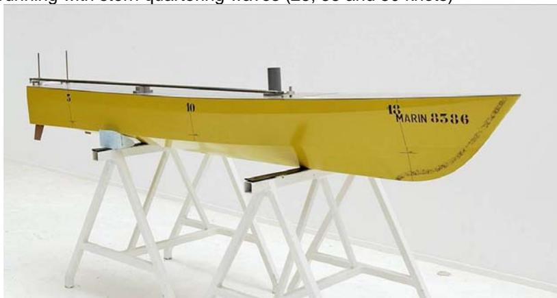
**Figure 5a: Model according to the Enlarged Ship Concept (ESC)**
